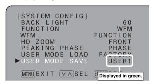
3 When the file whose data is to be saved is selected from the USER1 to USER5 files and the FUNCTION/ENTER button is then pressed, the screen shown below appears.
